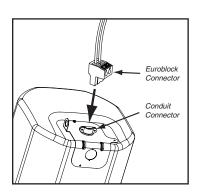
4. Loosen the conduit connector on the input terminal cover and insert wired euroblock the connector through the conduit connector opening. Connect the euroblock to the matching receptacle.
